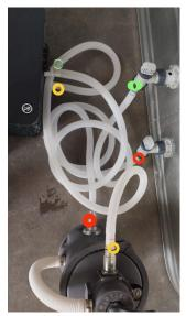
Connect the lowest inlet on the tank (red) with the lowest inlet on the filter pump (red). Use the clamps to tighten.
